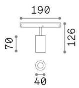
Net weight0.15 kgInsulation classIIIProtection indexIP20ComplianceCEOperating temperature $0^{\circ} \sim +40^{\circ}$
