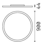
Net weight10.3 kgInsulation classIProtection indexIP40ComplianceCEOperating temperature $0^{\circ} \sim +40 \, ^{\circ}\text{C}$
