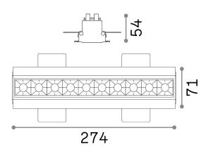
Net weight0.72 kgInsulation classIIProtection indexIP20ComplianceCEOperating temperature $0^{\circ} \sim +40 \, ^{\circ}\text{C}$
